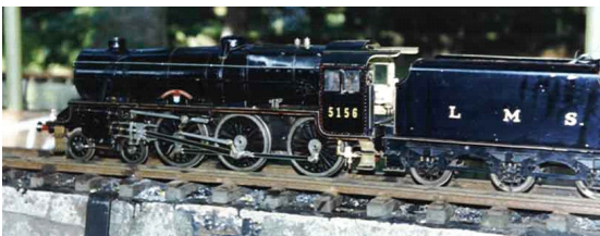
A 3 1/2" gauge 4-6-0 Stanier Black 5 model locomotive
