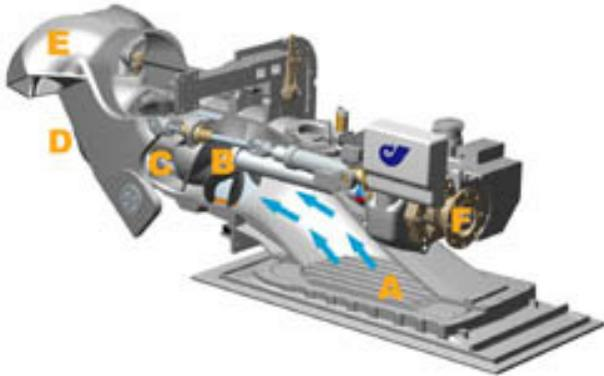
The picture below shows where water enters the jet unit via the Intake (A). The pumping unit, which includes the Impeller (B) and Stator (C), increases the pressure, or "head", of the flow. This high pressure flow is discharged at the nozzle (D) as a high velocity jet stream. The driveshaft attaches at the coupling (F) to turn the impeller.
