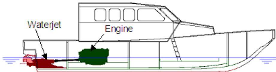
The hull of FCB2 will have no external appendages, apart from small bilge keels. This allows her to operate in depths that a traditionally driven propeller boat could not go.
