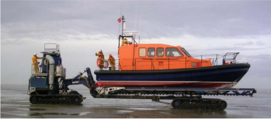
When FCB2 is safely on the carriage it is rotated by hydraulic power through 180° ready for the next launch. One of the many benefits of FCB2 launch and recovery is the saving on man (or woman!) power, especially during the recovery phase. To launch, only a Tractor Driver and Head Launcher are required, plus any Banksmen to ensure public safety. Recovery can be handled by smaller numbers too, as skids will not be needed in most cases.
