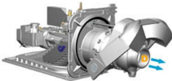
This reverses the direction of the force generated by the jet stream, forward and down, to keep the boat stationary or propel it in the astern direction.
