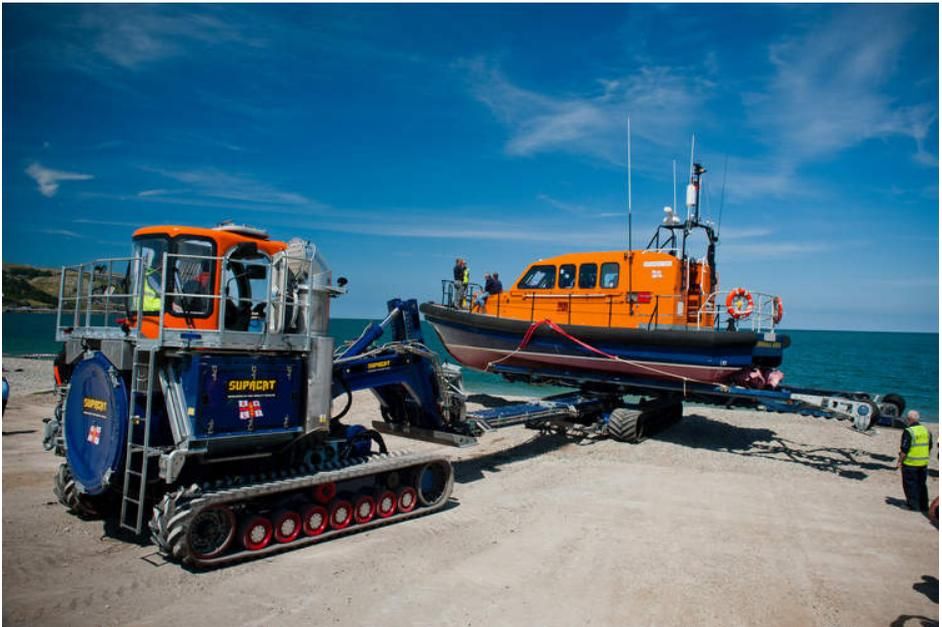
This first trial phase involves testing the alterations to the L&RS against diverse conditions at different stations, starting at Llandudno where an undulating and deep shingle bank cannot be negotiated using existing in-service launch systems, then Dungeness for its steep pebble beach, followed by Hoylake where spring tides mean distances of up 3 miles have to be covered from boathouse to water.
