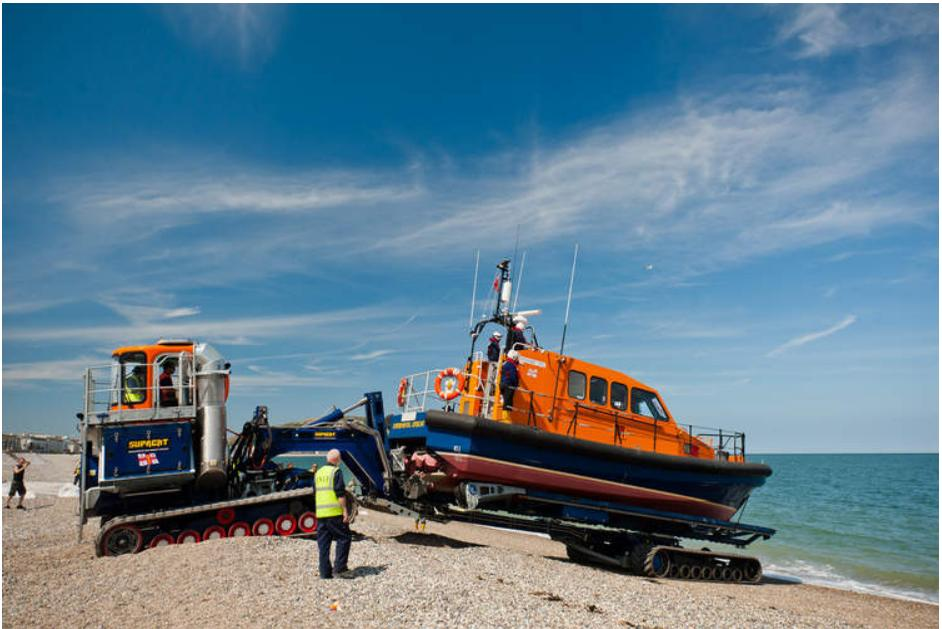
The L&RS is a track mounted, partially submersible tractor and powered-carriage system which has been custom designed by Supacat to launch and recover the new all weather lifeboat and carry it between the boathouse and water at stations where a harbour or slipway cannot be used.
